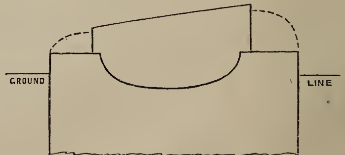
Fig. 2 shows a bed built as recommended, considerably wider than the frame, and not so high in the middle as at the sides, which gives two advantages—more room for earth, &c., and prevents so far a burning heat at the centre of the bed. These beds maintain a regular heat a long time, with the addition of the small linings at the top of the bed showed by the dotted lines. Of course, when the bottom heat gets too low, first one side of the bed and then the other is broken down, leaving enough for the security of the frame, and then the other side and the
